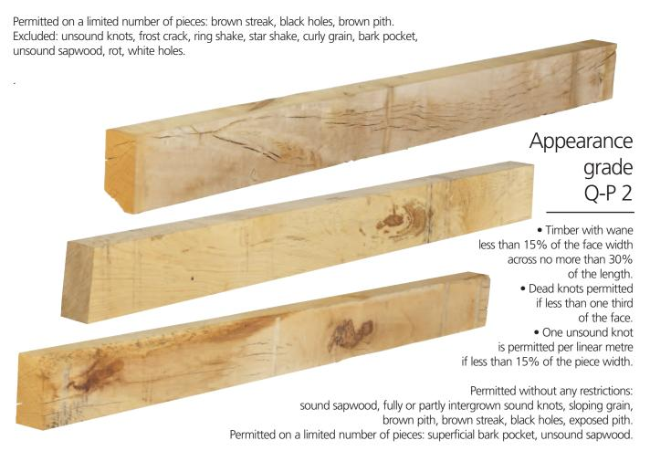
Excluded: frost crack, ring shake (unless it cannot be seen on the faces), rot, white holes.
